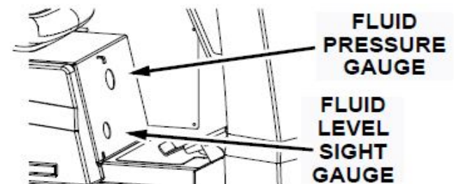
Fig. 3: Hydraulic Fluid Gauges
